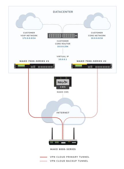
Mako-Mako Failover is not limited to data centre deployment, it can also be deployed (typically at edge locations or HQs) using any two Mako devices of the same type (e.g. 2 x Mako 6000-series Security Gateways).
