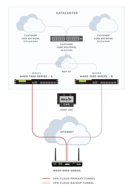
For example, each Mako VPN Concentrator can terminate connections from multiple VPN Clouds, with each Cloud treating that specific concentrator with a different priority.
