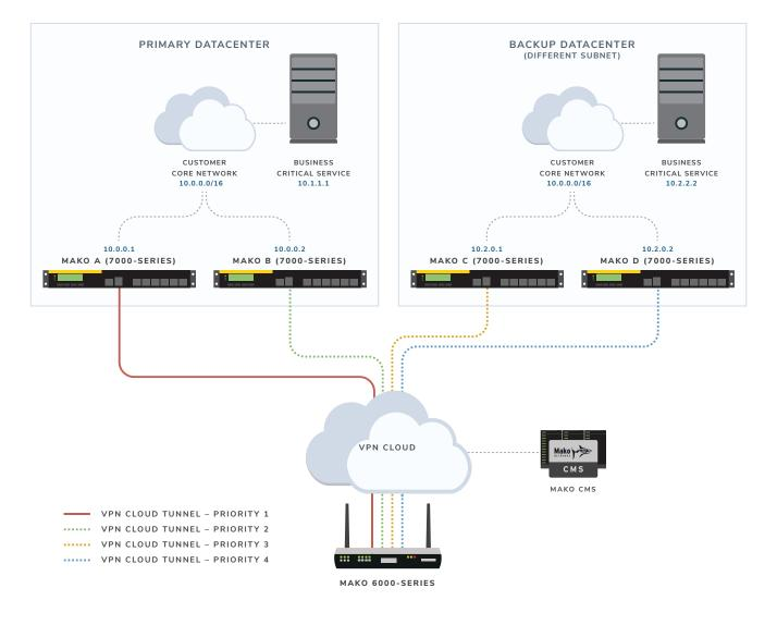
Alternatively, each data center can have unique addressing, with end-user applications configured to use the fallback addresses.
